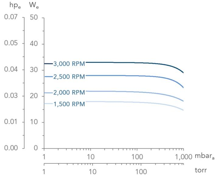
Flow Characteristics reflect nominal volume flow with air at NIST standard inlet conditions. Power Characteristics reflect nominal electric power consumption in Broomfield, CO USA with standard motor and controller losses.
